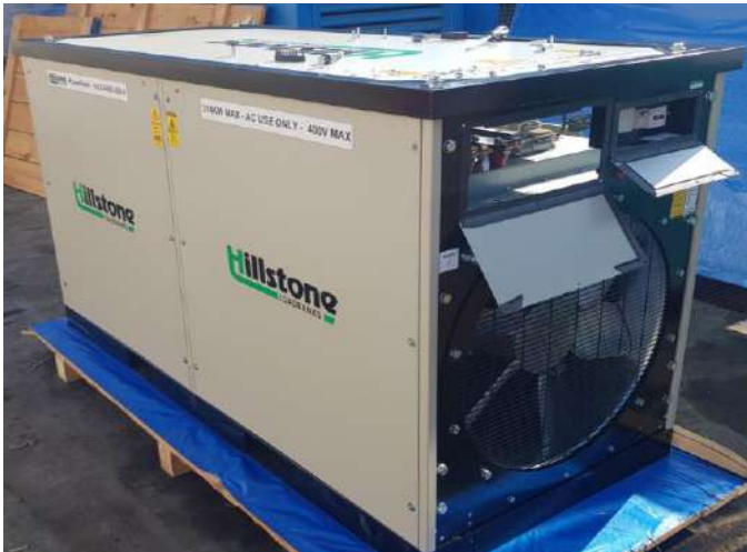
Figure 3. Hillstone load bank 3 phase AC, 400V, 319 kW
