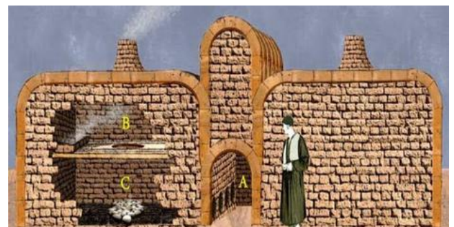
Figure 2. Egyptian incubator: A-the entrance to the incubator used for monitoring and maintaining the system; B-the area where eggs are placed for incubation, potentially elevated to optimize heat distribution; C-the lower chamber, which appears to house heat sources such as burning coals or materials to regulate temperature and humidity. The structure features chimneys or vents for ventilation and temperature control.
