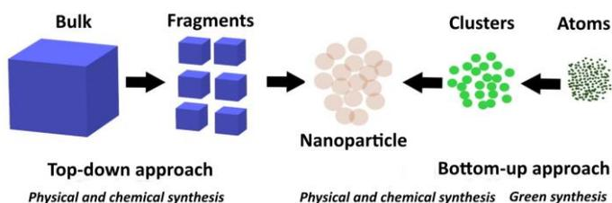
Figure 2. Nanoparticle's synthesis approaches [8]
