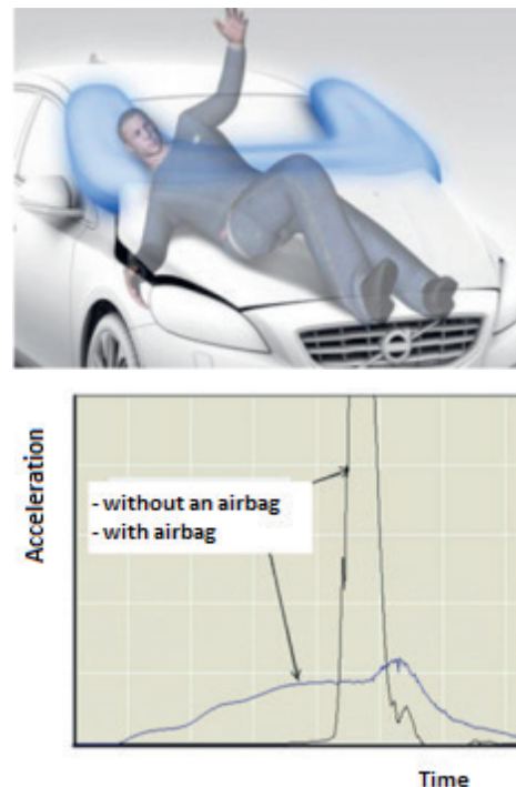
Figure 11. Acceleration of the head on the windshield, with and without an airbag
