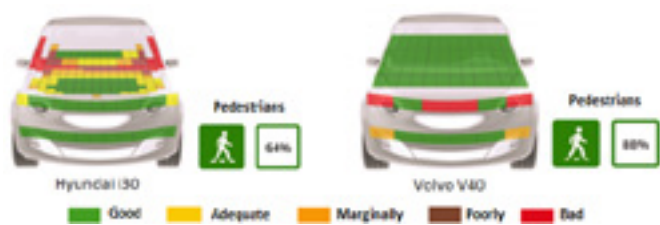
Figure 12. Assessment of pedestrian protection with and without an airbag
