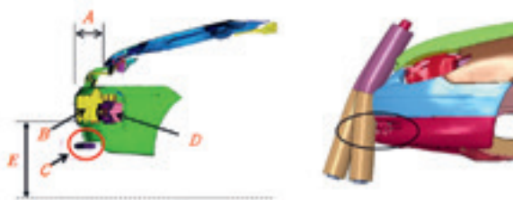
Figure 8b. The structure of the bumper and the shape of the collision between the leg and the bumper
