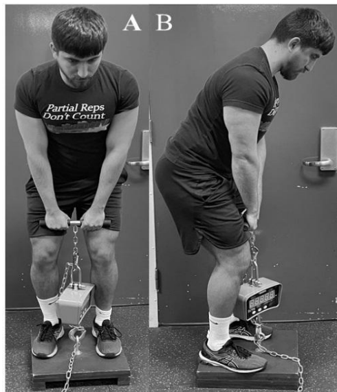
Figure 2. Frontal (A) and sagittal (B) view of the set-up for the adapted leg/back dynamometer test.
