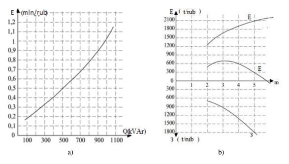
Fig.1. Functional dependences of price (a) and averaged efficiency (b) of high voltage PFC units use.
