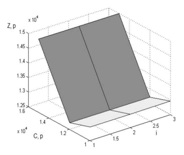
Fig. 2 Three-dimensional dependence of costs Z on the cost of static capacitors batteries and the number of its steps
