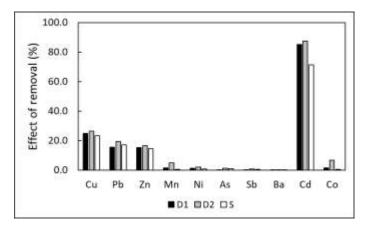
Figure 2 Comparison of effect of toxic elements removal from the soil by "10 M1" chelant in different dynamic and static conditions
