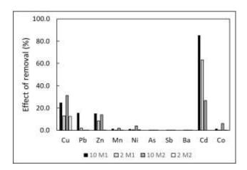
Figure 1 Comparison of effect of toxic elements removal from the soil by two studied chelants and in dependence on chelants concentrations
