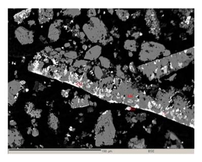
Figure 3 (left) BSE image of product obtained from the cathode after the electrolysis of effluent with "10 M1" chelant
