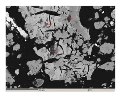
Figure 4 (right) BSE image of product obtained from the filtrate after the electrolysis of effluent with "10 M1" chelant
