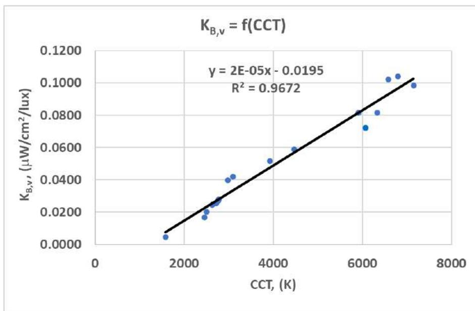
**Figure 9.** Graphical and defined linear analytical dependence of blue light hazard efficacy of luminous radiation  $K_{B,v}$  on the correlated colour temperature CCT of the measured domestic lamps
