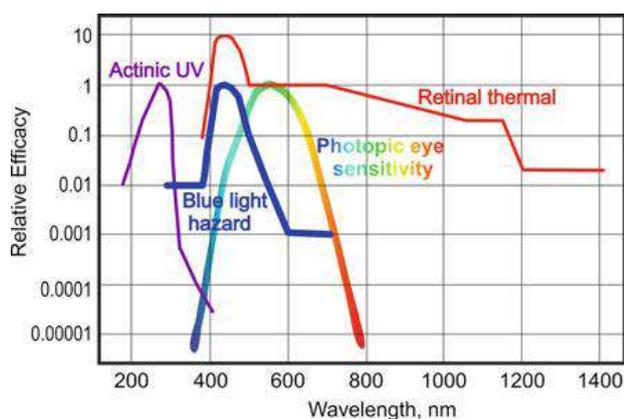
**Figure 1.** Photopic eye sensitivity, actinic UV, blue light and thermal hazards spectrums. [2]
