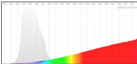
c) Dichroic halogen lamp-15W
