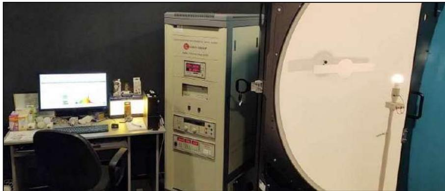
Figure 3. Measurement of the spectral emission of the studied domestic lamps with a CCD spectroradiometer system
