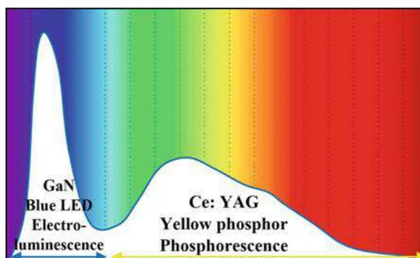
**Figure 2.** Spectrum formation of Blue LED + Yellow phosphor technology LEDs
