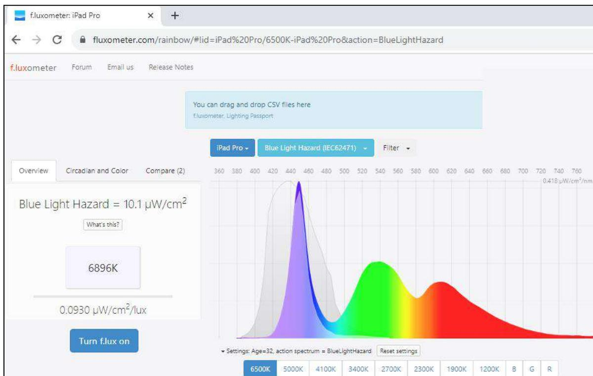
Figure 6. Online application and service f.luxometer™ used to process the spectral power distribution data in CSV format
