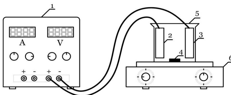
**Figure 1.** Scheme of electrocoagulation process setup: 1 – source of electric power; 2 – anode; 3 – cathode; 4 – magnetic stir bar; 5 – electrochemical cell; 6 – magnetic stirrer
