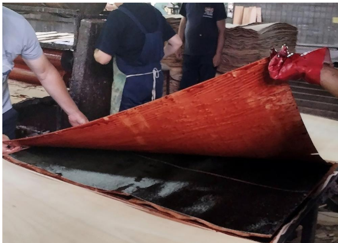
Figure 1. RLVL construction assembly for PF adhesive combination ( F_{kl} )
