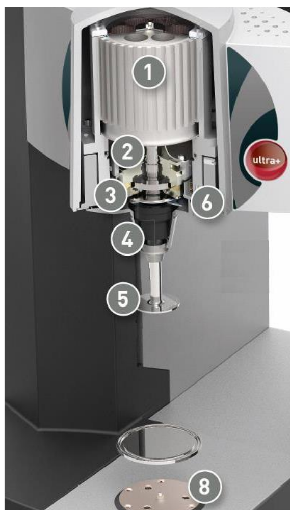
Figure 4. Thermo Scientific HAAKE MARS iQ Rheometer Air-bearing Principles –Measurement 1. Drag Cup Motor = Stress, 2. Air Bearing; 3. Position Sensor = Shear Rate (Strain); 4. Geometry Recognition & Chuck; 5. Measurement Geometry / Measuring System; 6. Strain Gauge = Normal Force & Automatic Gap; 8. Temperature Control
