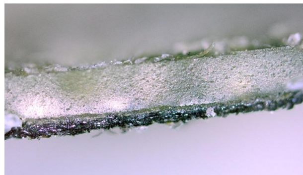
Figure 3. Optical image of cross-sectional PU–MXene composite (100× magnification).
