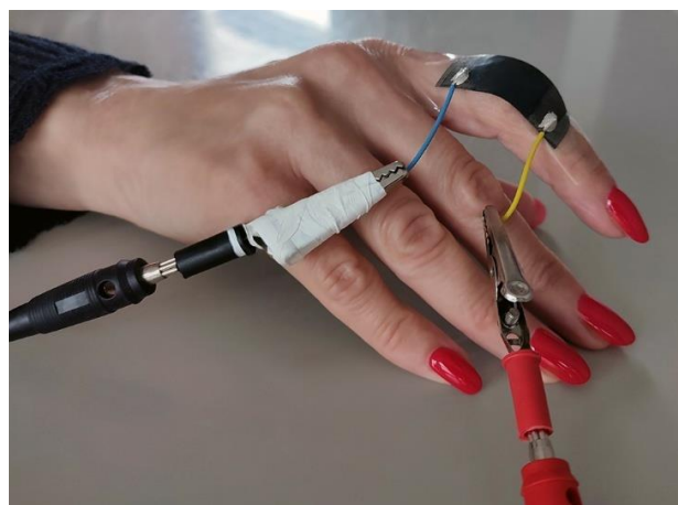
Figure 4. Photograph of MXene sensor during finger flexion.
