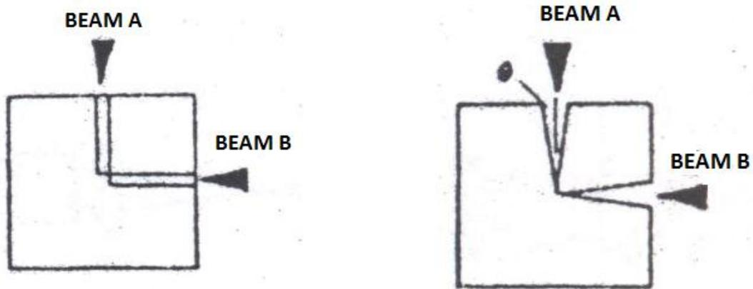
Figure 3. Machining using two laser beams
