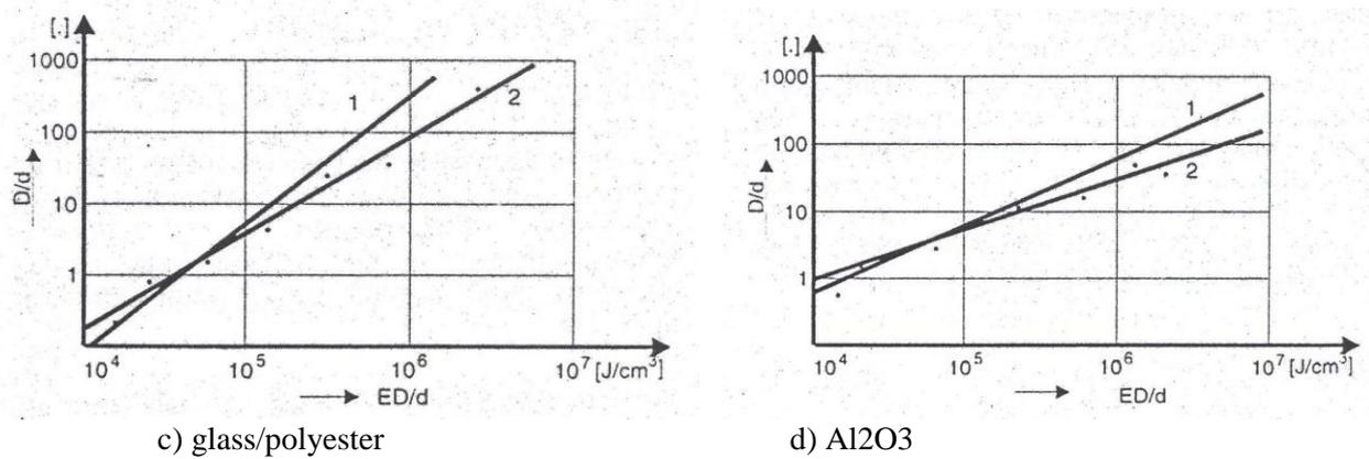
Figure 5. Comparison of computing (1) and experimental (2) results for glass/polyester (5c) and Al<sub>2</sub>O<sub>3</sub> (5d)
