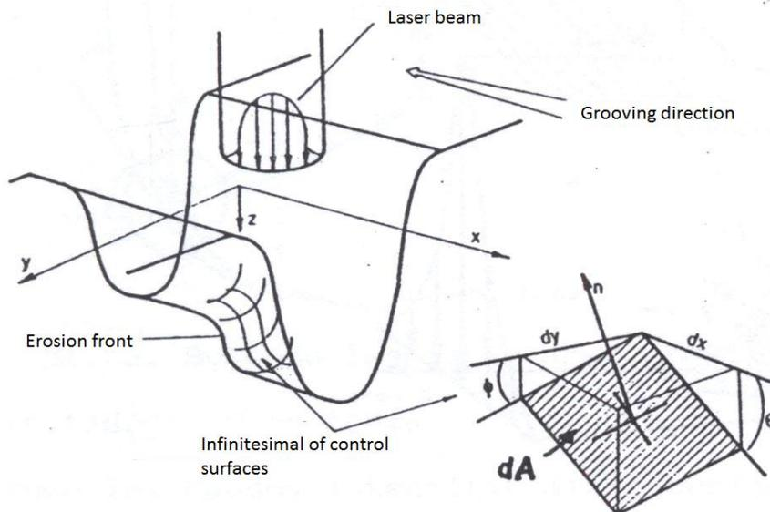
Figure 1. Creation of a groove using one laser beam
