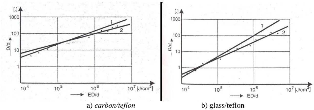
Figure 4. Comparison of computing (1) and experimental (2) results for carbon/teflon (4a) and glass/teflon (4b)
