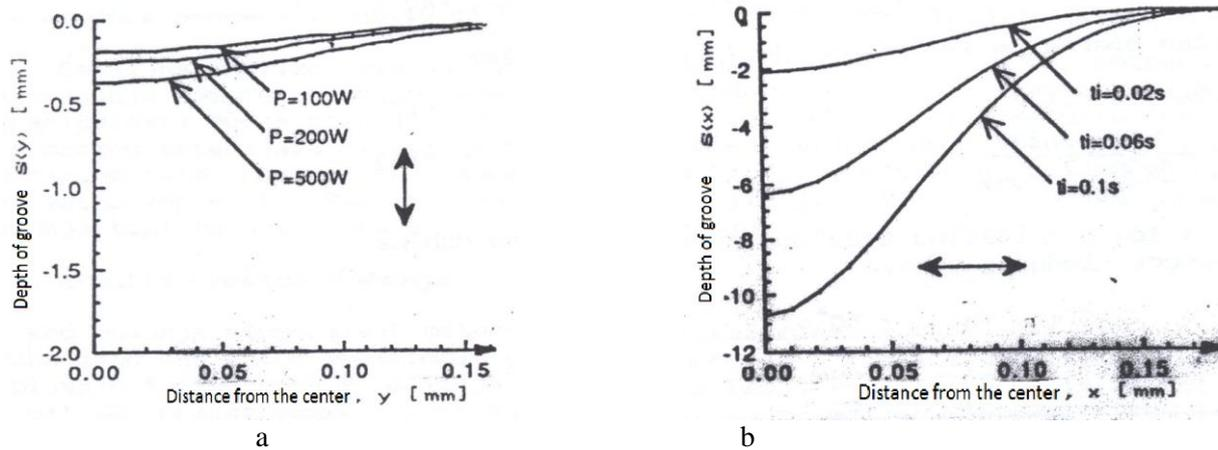
Figure 6. Depth of the laser beam penetration: a) axial to the fibres; b) radial to the fibres
