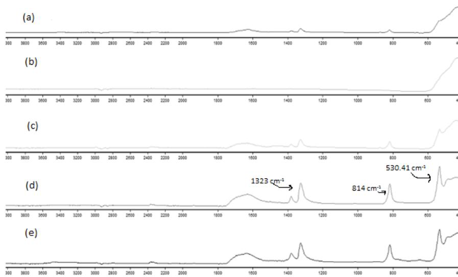
Figure 1. FTIR spectra of ZnO nanoparticles synthesized using different amount of glycerol as a dispersant, designated with following order (sample 1 - a, sample 2 - b, sample 3 - c, sample 4 - d and sample 5 - e)
