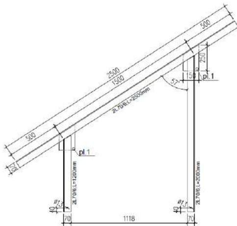
Figure 1-a). Roof metal construction for the photovoltaic power plants
