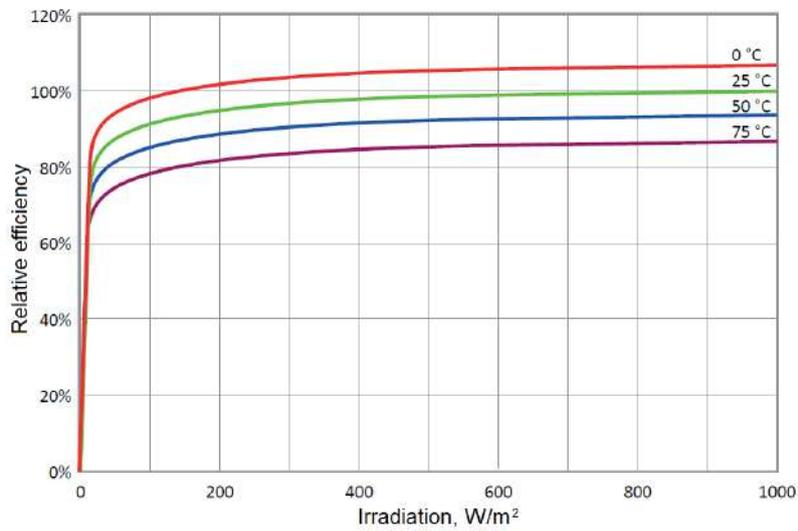
Figure 6. Performance at different cell temperatures of the CdTe PV module 100 Wp
