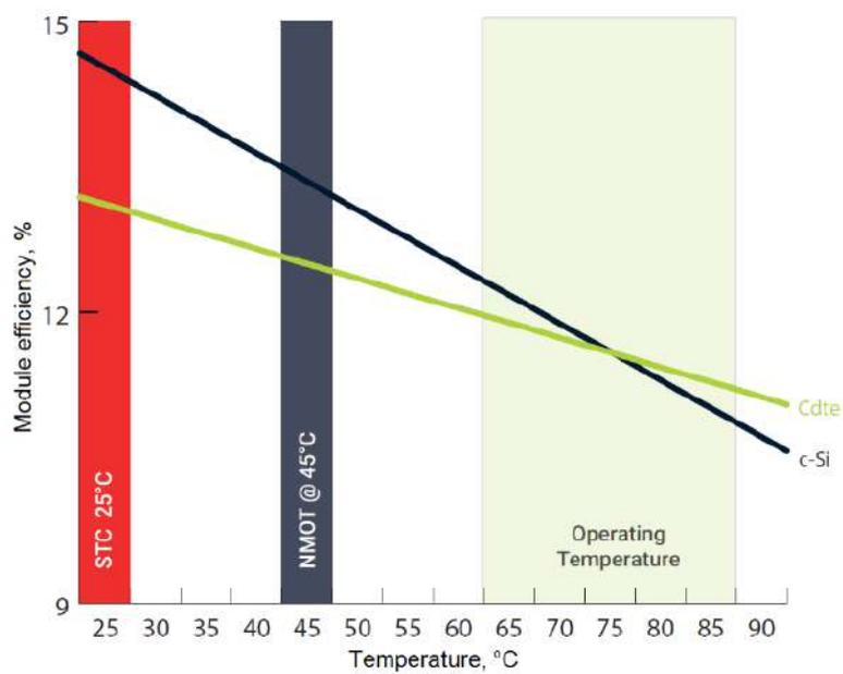
Figure 7. Comparative efficiency at different PV cell temperatures between CdTe and crystalline silicon material
