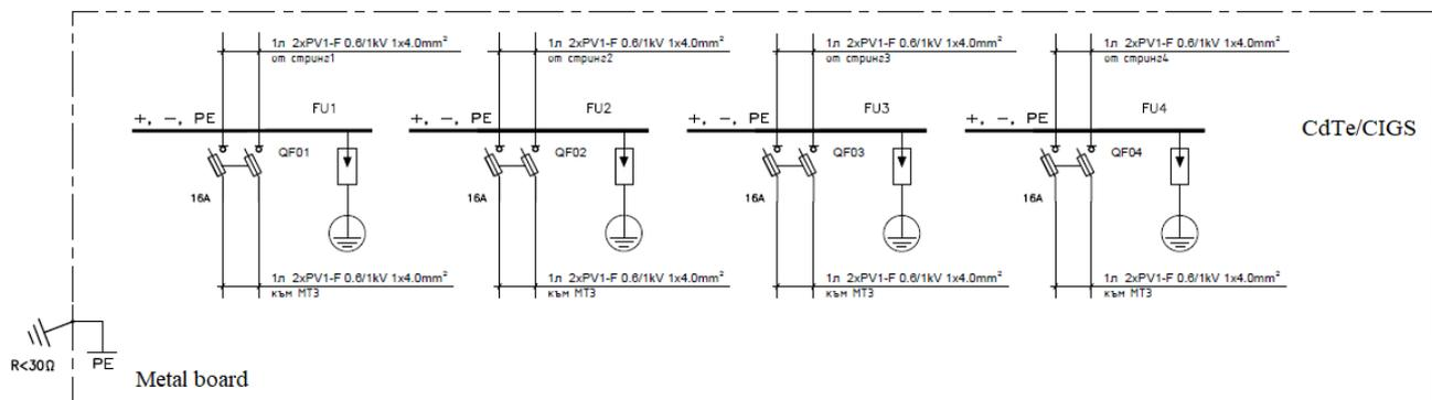
Figure 13. Schemes describing basic wiring diagram of the individual strings for CdTe and CIGS PV module
