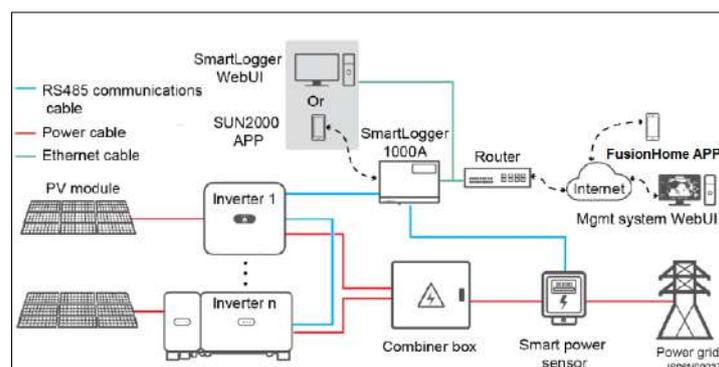
Figure 15. Communications with inverters by access over a local ethernet and Wi-Fi
