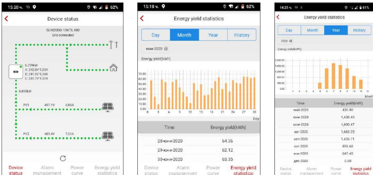
Figure 16. Communications with inverters SUN2000-10KTL-M0 over Wi-Fi with FusionHome App
