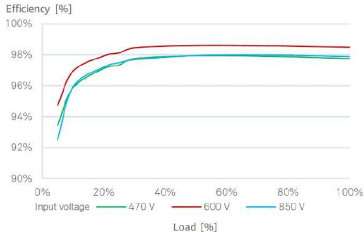
Figure 12. Efficiency curves of the inverters SUN2000-10KTL-M0 at different input voltage
