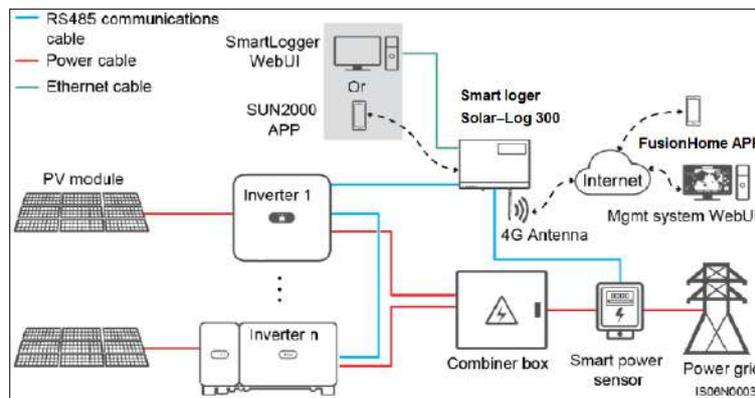
Figure 14. Communications with the inverters and smart logger by access over a public network
