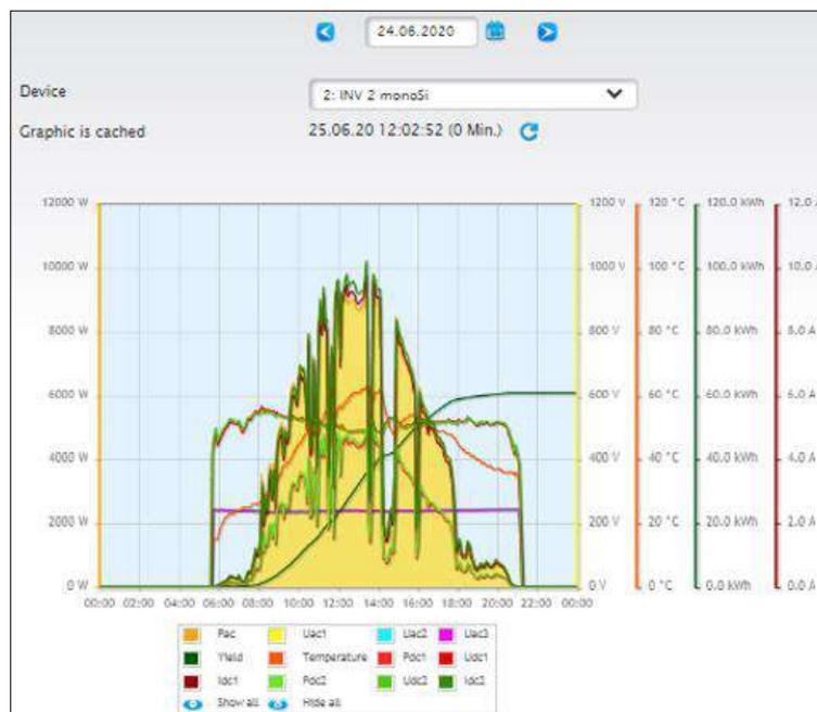
Figure 19. The inverter details of the mono-Si PV modules power plant
