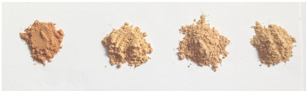
Figure 3. Photography of N-ion doped ZnO calcined at (from left to right) 300, 400, 500, and 600 °C
