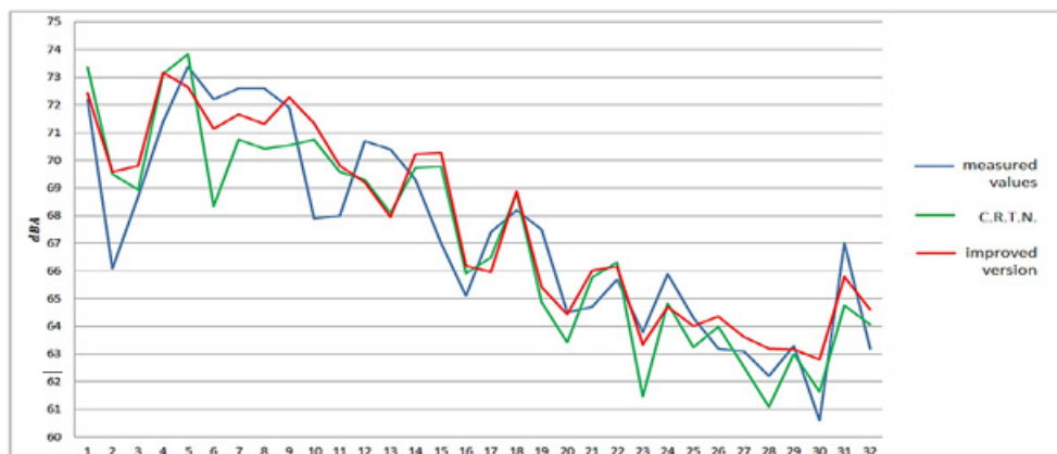
Chart 1: Display of the relation between measured, predicted and calibrated values for C.R.T.N. model
