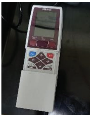
Figure 2. Device used to measure the roughness Mitutoyo SJ-210
