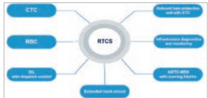
Fig. 6. RTCS subsystem composition
