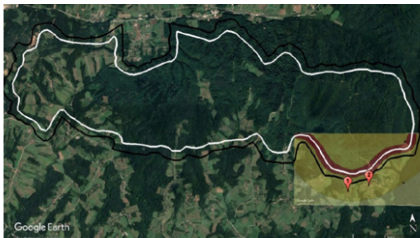
Figure 10. The fifth examined segment of the mine front of 2645 m length, with proposed measuring points, next to residential buildings near the mine, potentially most affected by noise
