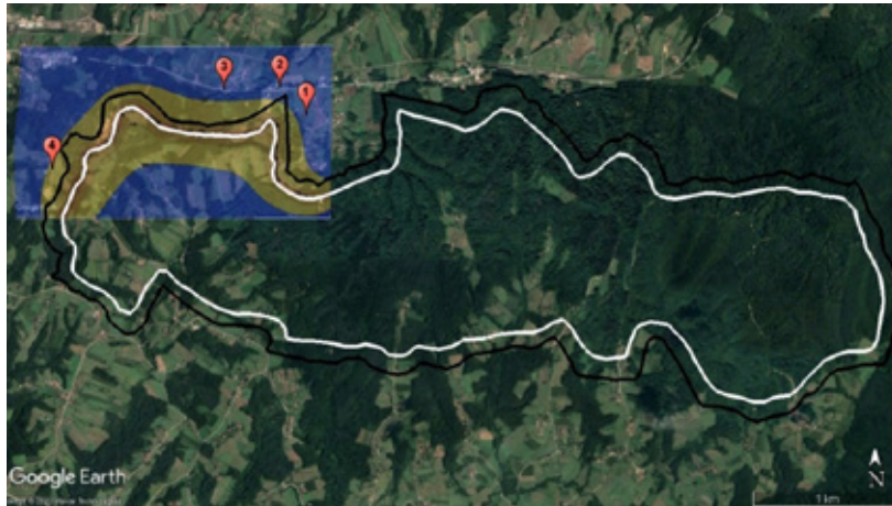
Figure 4. The second examined segment of the mine front of 2938 m length, with proposed measuring points next to residential buildings near the mine, potentially most affected by noise
